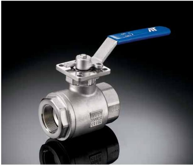
Triac Series 24 High Pressure Ball Valves feature a high quality investment cast body and end. They are available in 1/4" through 2" (all are full port except the 2" size). Superior leak protection is accomplished by using our patented Pyramidal Stem Seal Packing System shown in the graphic below. This advanced system protects against wear and leakage experienced by other ball valves.
